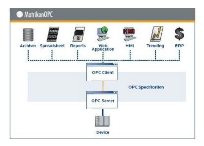
This standardized data exchange between the OPC Clients and OPC Servers allows any OPC Client to communicate with any other OPC Server. Since the OPC Server takes care of translating Native device communications into an OPC format and the OPC Client does the same on the Application side; Applications and Devices can share data between each other without having to know each other's native protocols or data formats.
