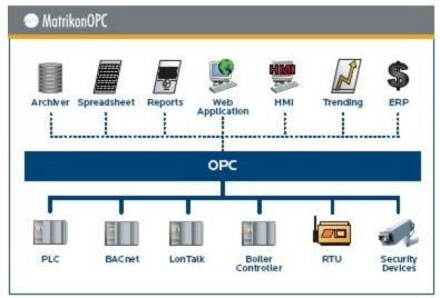
OPC Specifications define how OPC Clients and OPC Servers communicate but leave the OPC Client-Application and OPC Server-Device communications open since this depends on the Application and Devices being used.
