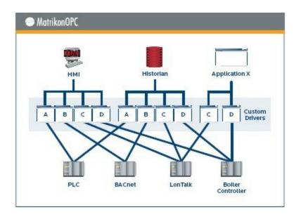
OPC offers a simple, standards based, solution for this problem. It introduces an abstraction layer between devices and applications to allow data to pass between them without them being aware of each other's internal data representations.
