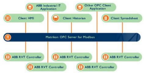
The schema shows five RVT controllers (Power Factor controllers) as Modbus slave devices connected to the Matrikon OPC Server for Modbus. Different OPC Clients can interact with the OPC Server.
